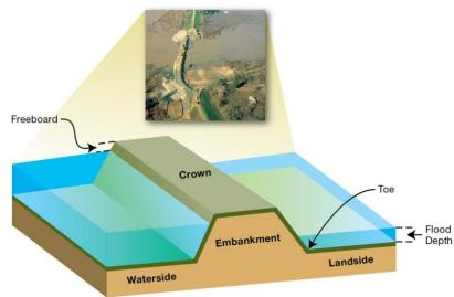
Figure 4.4 – Components of a Typical Levee
